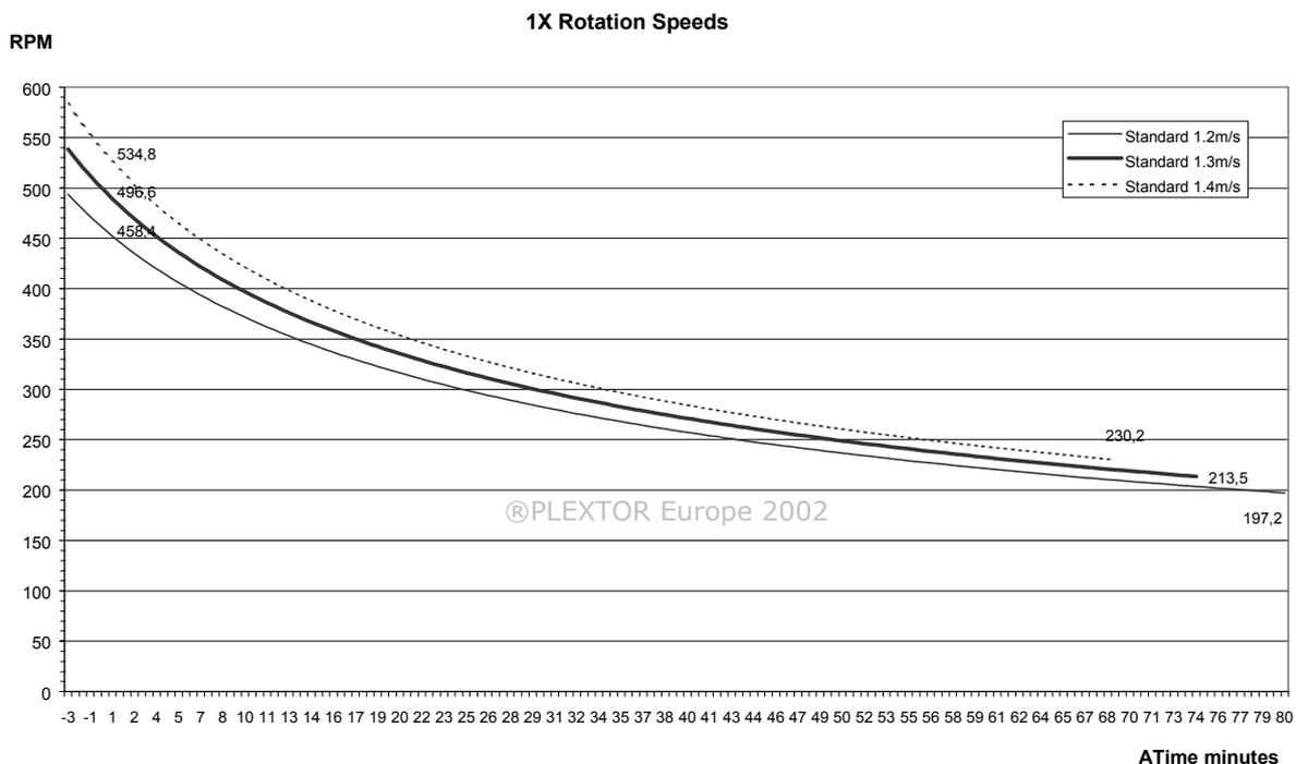
When we want to increase the write speed, we have to take into account the physical limitations of the drive. Depending on the mechanism used in the drive, a limitation of 9200 to 9600 RPM is set. Above this speed, it will become too difficult to control vibration of the disc and establish correct positioning, what may result in write errors or playback problems.
