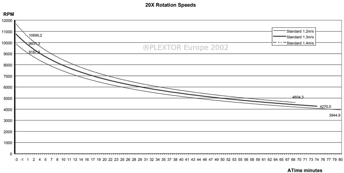
When Z-CLV is used, the switch points to the higher speeds are precisely calculated to allow the speed in the next zone to start at the same RPM again (this is media dependent). Therefore the switching points in Plextor Recorders are not fixed, but greatly dependent on the media that is being used as you can see on the next graph.
