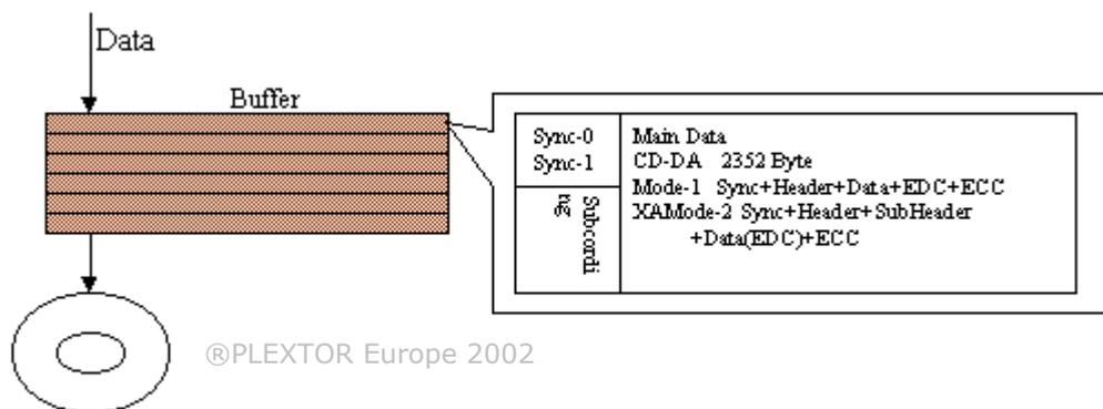
This buffer then serves to bridge over minor interruptions in the data stream from the PC. Under normal conditions, the data buffer should always be capable of holding enough data to guarantee smooth recording.
